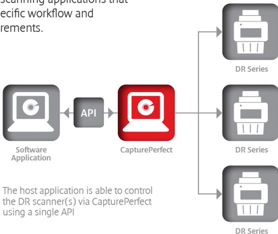
The host application is able to control the DR scanner(s) via CapturePerfect using a single API
