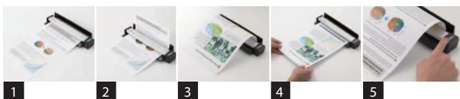
**1** Insert the page face up and press the Scan button. **2** The S1100 proceeds to scan the front side. **3** The page exits facing front side down. **4** Reinsert the page without pressing the Scan button. **5** The page is scanned. Press the Scan button to end the scanning process and create the PDF image file.
